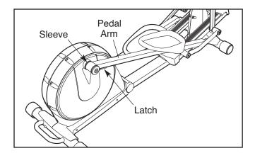
Next, raise the pedal arms until they touch the magnets on the upper body legs; the magnets will hold the pedal arms in place. Then, hold the handle and lift the frame until it locks in a vertical position.
